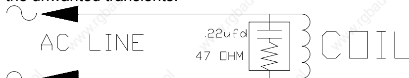
Figure 3.2 AC Coil Suppression
