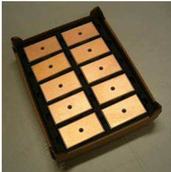
Fig. 9.2 – ESD blister with module inside
