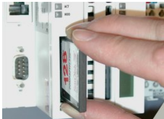
FIG2: Removing the CF card
