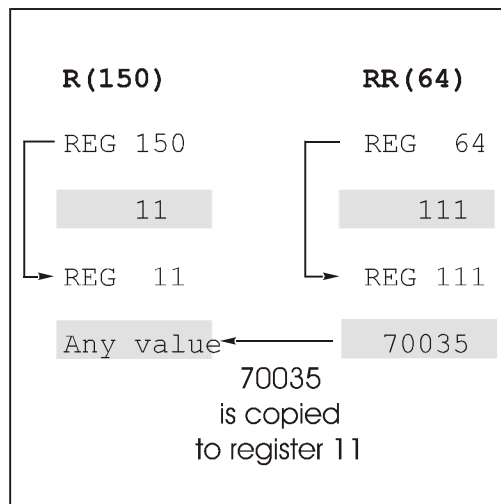
Fig. 21: Example for Double Indirect Addressing
