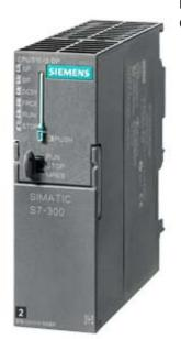
SIMATIC S7-300, CPU 315-2DP CPU WITH MPI INTERFACE INTEGRATED 24 V DC POWER SUPPLY 256 KBYTE WORKING MEMORY 2. INTERFACE DP-MASTER/SLAVE MICRO MEMORY CARD NECESSARY
