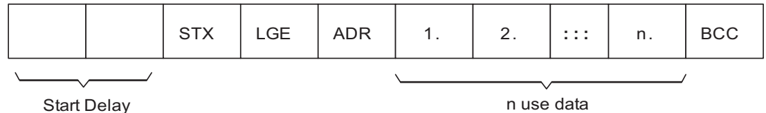
Figure 6-18 Structure of USS telegram
