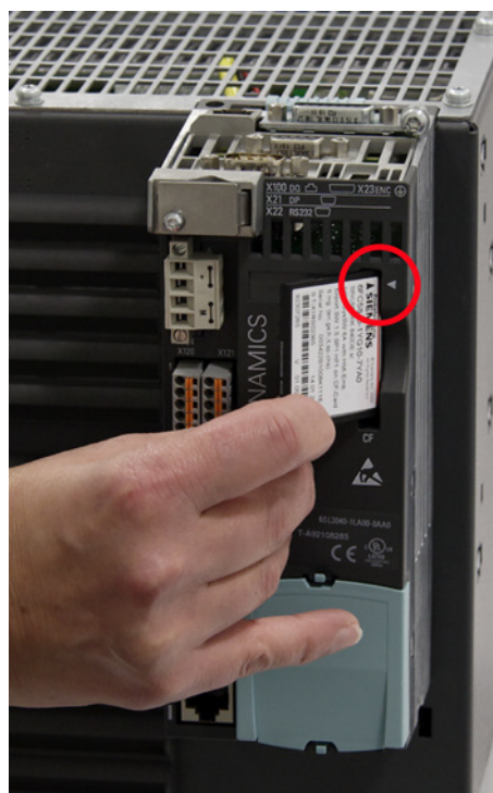
Figure 7-12 CU310-2 DP Inserting the memory card
