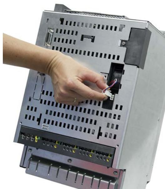
4. Withdraw the connector. To do so, gently press the interlock and connector together.
