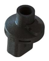
For improved air filtration system performance, the NovaSensor FMA Series of Filtration Air Restriction (FAR) Sensors accurately measures pressure loss across a variety of air filtration devices utilizing high accuracy NPA piezoresistive technology in a low-profile form factor that is easy to install and maintenance-free.
