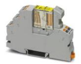
Pre-assembled relay module with Push-in connection, consisting of: relay base, safety relay with force-guided contacts in accordance with DIN EN 50205, plug-in display/interference suppression module, and retaining bracket, contact type: 2 changeover contacts, input voltage: 24 V DC
