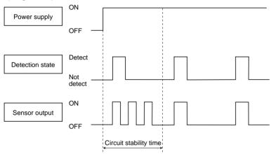
Remark: Circuit stability time: 45s max. (45s max. for the 10m detection type)
