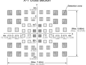
Remarks: 1. The X-Y cross-sectional diagram shows the detection area. 2. The differences in the detection zone patterns are indicative of the projections of the 16 lenses with single focal point and with five optical axes. An object whose temperature differs from the background temperature and which crosses inside the detection zone will be detected.
