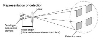
3. Lenses can be miniaturized because the pyroelectric element is small
