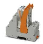
Pre-assembled relay module with screw connection, consisting of: relay base, power contact relay, and retaining bracket. Contact type: 3 changeover contacts. Input voltage: 24 V DC
