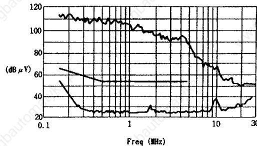
European Standards EN55011 Class B measurement data
