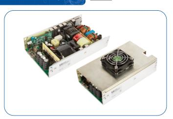
The Class II PBL500 series of AC-DC switching power supplies, in a package of just 4 x 7 x 1.56 inches, deliver 450-500 watts of continuous power with forced air cooling or 250 watts with convection cooling. The units are constructed on a U-Channel for mechanical support and heat sinking. A cover and fan assembly can be added during manufacturing. They are designed for medical applications including those needing BF rated insulation with an operation altitude up to 5000 meters.
