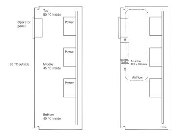
In most cases, the ambient temperature for the operator panel is significantly higher than the device cabinet's ambient temperature.
