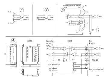
Some (older) operator panels had pull-up and pull-down resistance except for the actual bus termination at 120 ohm, similar to Westermo and Profibus. See 1 in drawing above.
