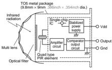
• Block diagram of the analog output circuit
