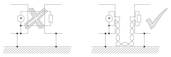
Figure 4: Cable laying - loop area
