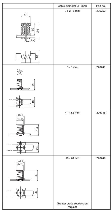
Figure 8: Screening terminals for grounding
