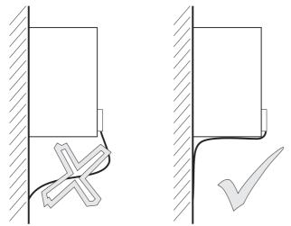
Figure 3: Cable laying - aerial height
