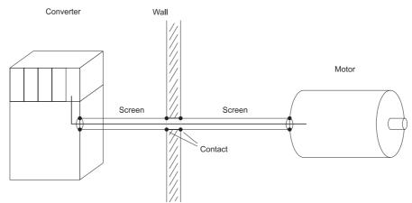
Figure 5: Cable laying - cabinet outlet
