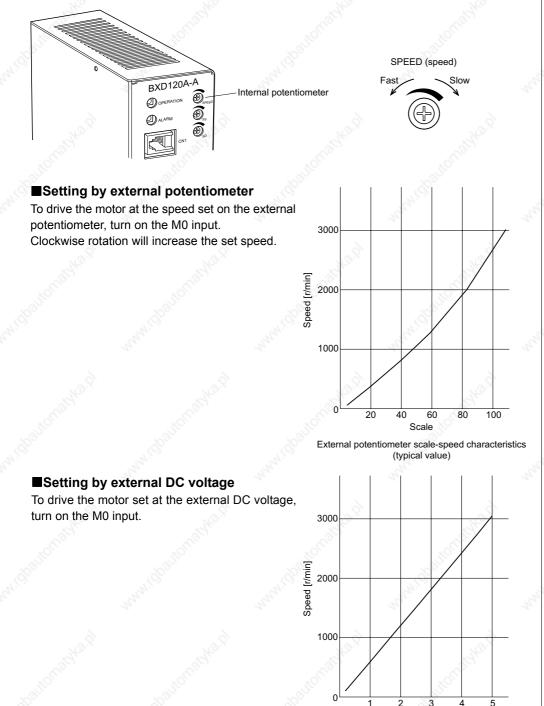
External DC voltage [V] External DC voltage-speed characteristics
