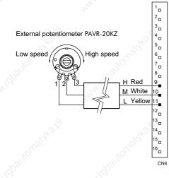
To connect the external potentiometer, use the attached external potentiometer and the signal cable [1 m (3.3 ft.)] for connection of the external potentiometer.
