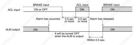
You can reset the protection function by cycling on the power supply. Be sure to turn on power again after removing the cause for the operation of protection function; then reset ALM output.
