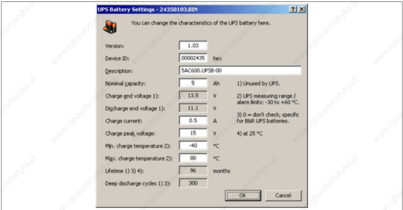
Figure 160: ADI Control Center - UPS battery settings
