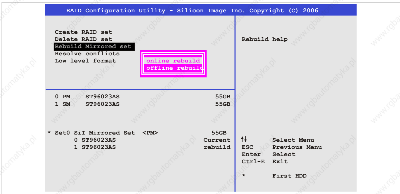
Figure 109: RAID Configuration Utility - Rebuild mirrored set
