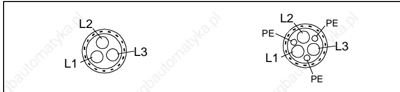
Figure A-2 Recommended motor cables.
