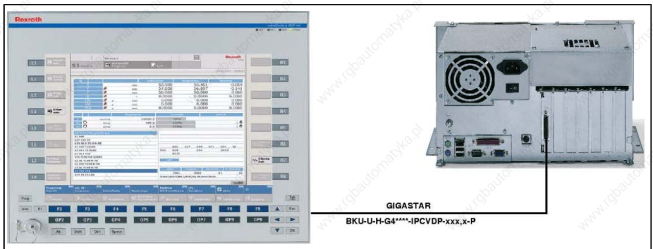
Fig.7-2: VSB 40 standard industrial PC with VDP 40 operator panel
