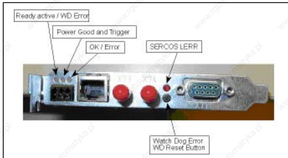
Fig.4-6: LEDs and external watchdog reset button
