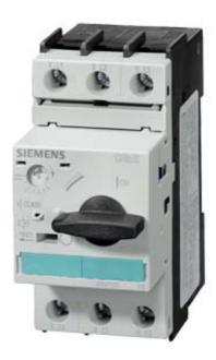
CIRCUIT-BREAKER SIZE S0, FOR MOTOR PROTECTION, CLASS 10, A-REL. 20...25A, N-REL. 325A, SCREW TERMINAL, STANDARD SWITCHING CAPACITY
