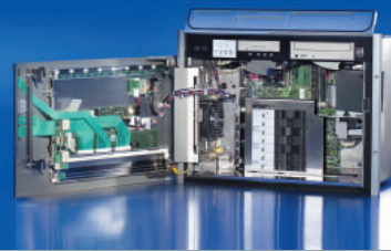
If the front door is open, it is possible to access all the components.
