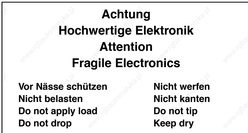
Fig 16.1: Guidelines on storage and transport on packaging
