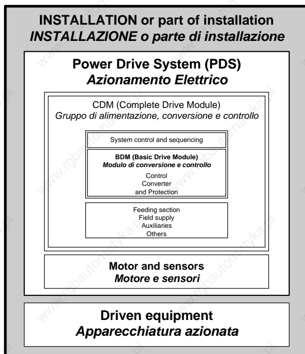
Fig. 1-1: Block diagram of the installation and the power drive systems (PDS)
