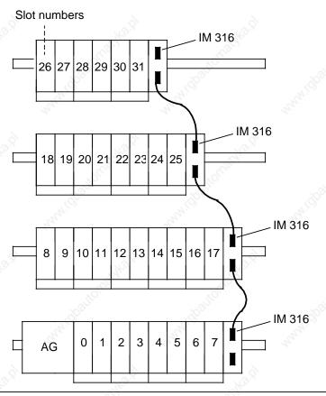
Figure 6-3. Slot Numbering in a Multi-Tier Configuration
