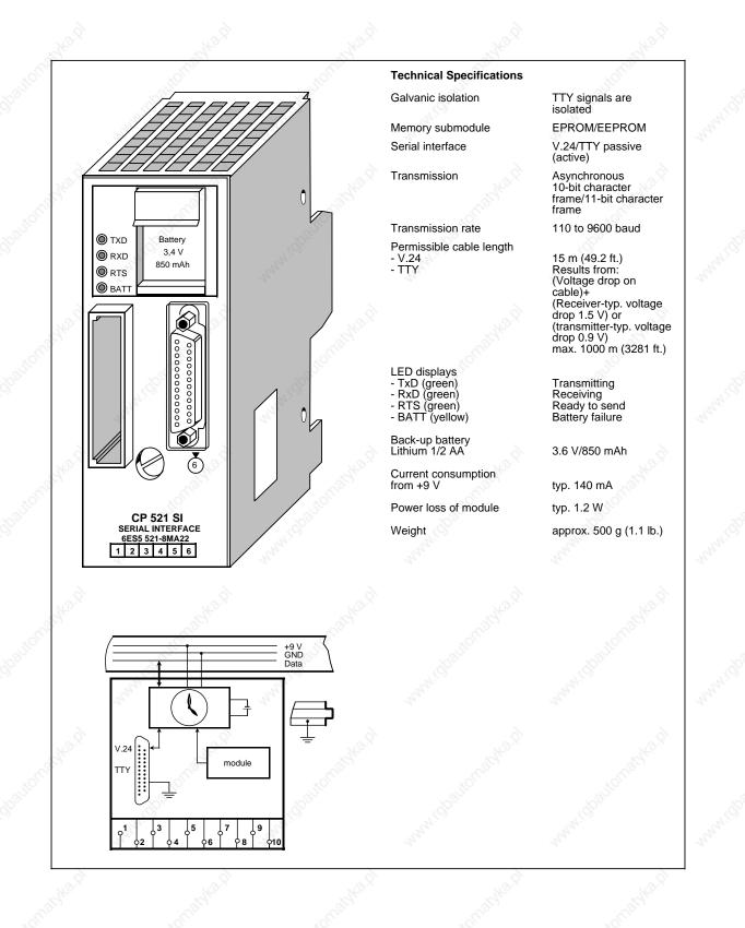
The CP 521 SI (Serial Interface) communications module is a powerful I/O module with its own central processor.
