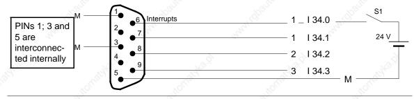
Figure 3-24. Connecting the Interrupt Inputs
