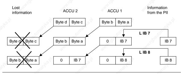
Figure 8-2. Execution of the Load Operation
