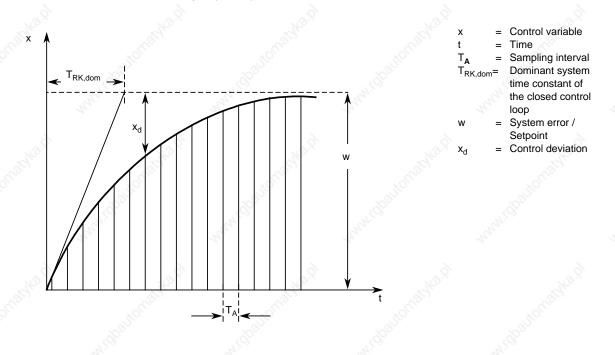
Figure 9-5. Principle of Interval Sampling
