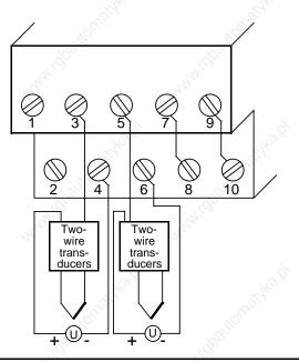
Figure 15-11. Connection of only Two-Wire Transducers (6ES5 464-8MD11)
