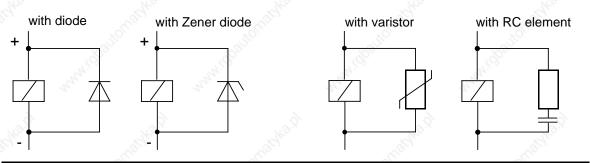
Figure 3-33. Wiring Coils
