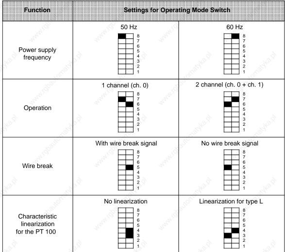
Table 15-28. Settings for the Operating Mode Switch for Analog Input Module 464-8MF21
