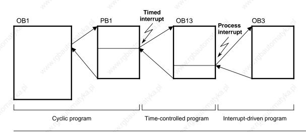
Figure 9-1. Time-Controlled Program Execution - Possible Interrupts
