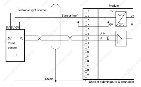
If there is no sensor line between the sensor and the counter module, pins 1 and 2 of the module must be bridged.
