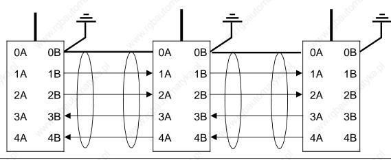
Figure 14-2. Connection of the Bus Cable
