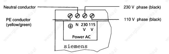
Figure 3-17. Connecting the S5-90U to the Supply Mains
