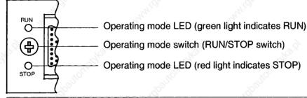
Figure 4-1. Operator Panel of the S5-90U
