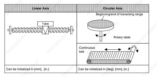
Figure 16-28. Processed Units of Measurement for Circular Axis and Linear Axis
