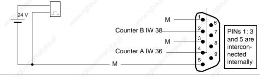
Figure 3-25. Connecting a Counter Input
