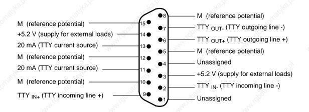
Figure 2-2. Pin Assignments of the Programmer Interface of the S5-90U
