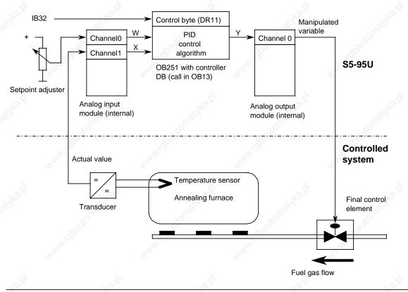
Figure 9-6. Process Schematic
