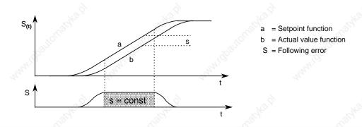
Figure 16-29. Course of a Following Error during a Positioning Operation
