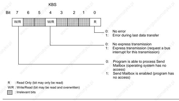
Figure 14-6. Structure of the Coordination Byte Send (KBS)
