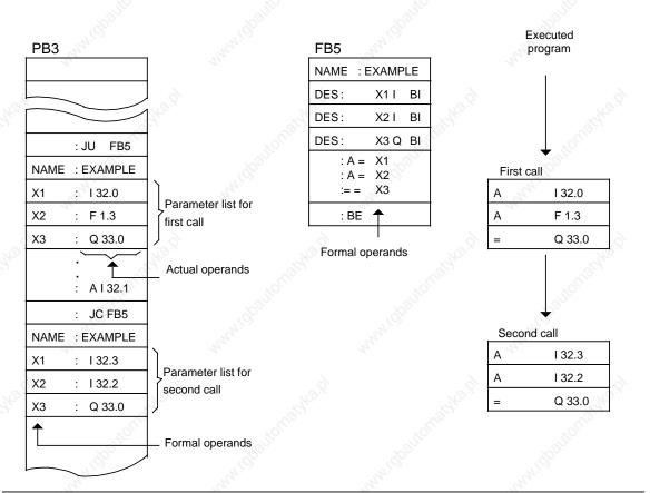
Figure 7-5. Programming a Function Block
