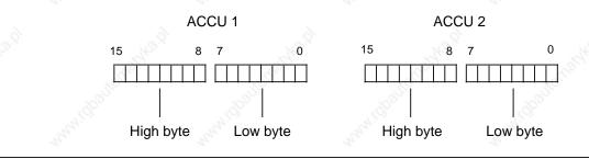
Figure 8-1. Accumulator Structure
