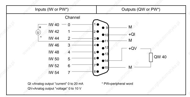
Figure 3-23. An Example of an Analog Input and an Analog Output Connection
