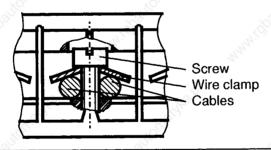
Figure 3-14. SIGUT Screw-Type Connection
