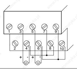
Figure 15-17. Wiring Possibilities for ±500 mV Voltage Measurement for the Input Module (6ES5 464-8MF11)
