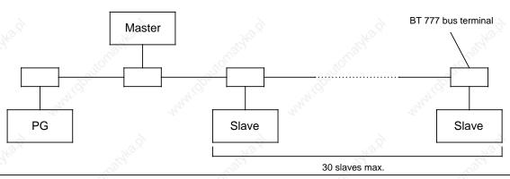
Figure 14-1. Structure of a SINEC L1 LAN
