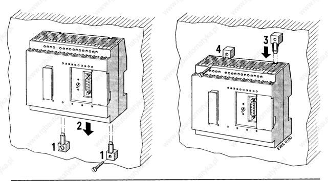
Figure 3-1. Mounting the S5-90U on a Wall
