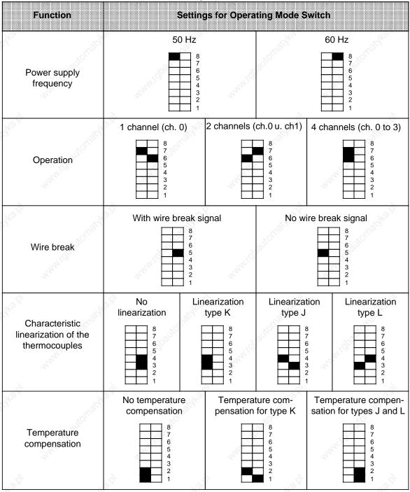
Table 15-12.Settings for the Operating Mode Switch<br/>for Analog Input Module 464-8MA21
