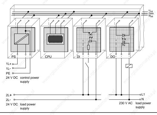
Figure 3-30. Simplified Representation for Installation with Floating Modules
