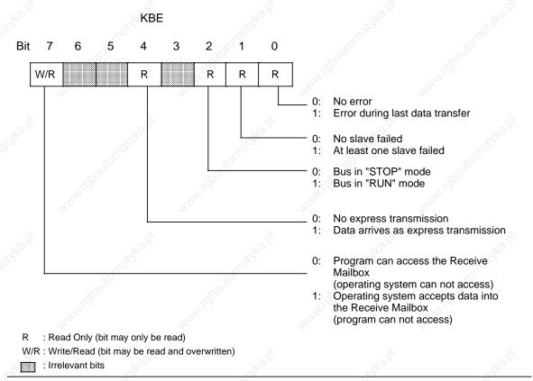
Figure 14-8. Structure of the Coordination Byte Receive (KBE)
