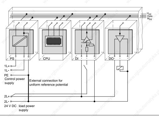
Figure 3-29. Simplified Representation of an Installation with Non-Floating Modules
