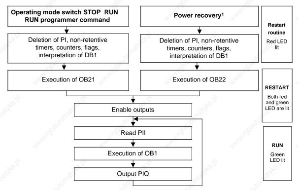
1 If PLC was switched to RUN at POWER OFF; if operating mode switch was set to RUN at power recovery and battery backup was provided. Without battery backup, a memory submodule containing valid blocks must have been inserted.
