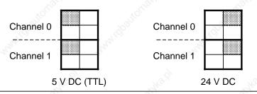
Figure 16-5. Setting the Input Voltage Range on the Counter Module (500 Hz)
