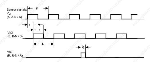
Figure 16-14. Signal Sequence for Up-Counting
