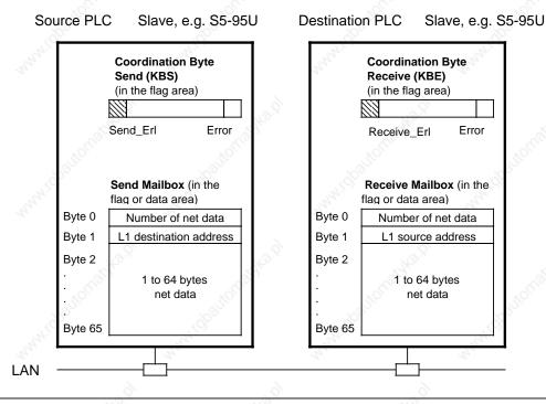
Figure 14-3. Principle of Data Interchange
