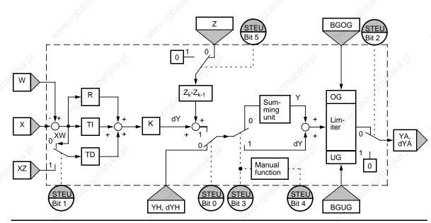
Figure 9-4. Block Diagram of the PID Controller
