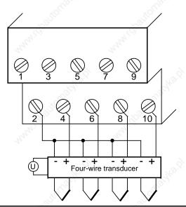
Figure 15-14. Connection of only Four-Wire Transducers (6ES5 464-8ME11)
