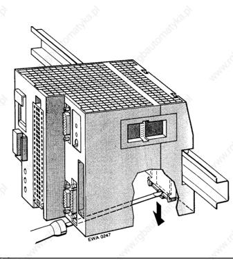
Figure 3-4. Removing the Programmable Controller
