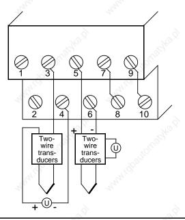
Figure 15-12. Connection of Two-Wire and Four-Wire Transducers (6ES5 464-8MD11)
