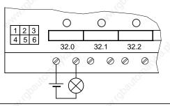
Figure 3-20. Example of How Digital Outputs Can Be Connected
