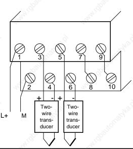
Figure 15-13. Connection of only Two-Wire Transducers (6ES5 464-8ME11)
