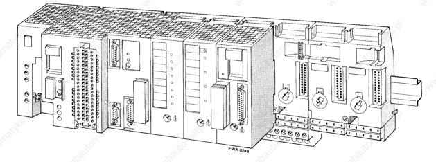
Figure 3-7. Installation with External I/Os for an S5-95U
