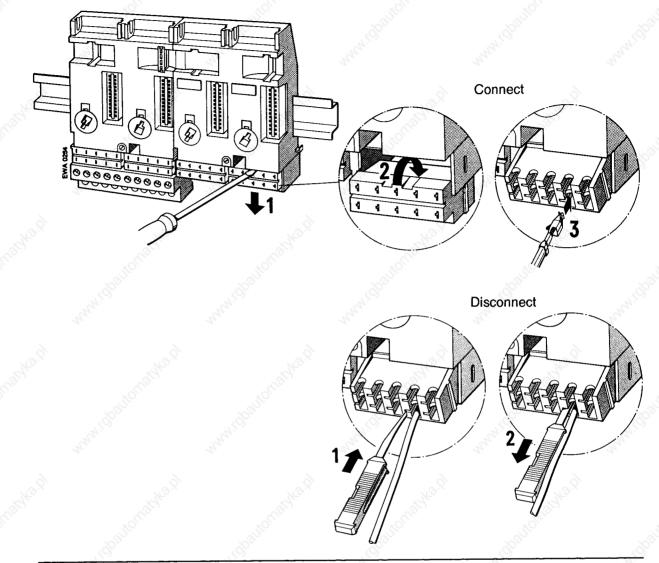
Figure 3-16. Connecting and Disconnecting Crimp Snap-In Contact
