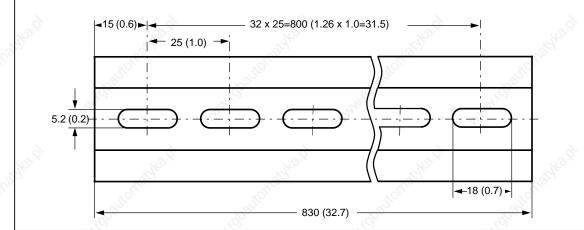
Figure C-4. Dimension Drawing of the 830-mm (32.7-in.) Standard Mounting Rail
