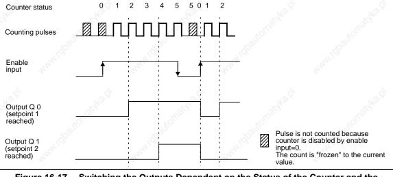
Figure 16-17. Switching the Outputs Dependent on the Status of the Counter and the Enable Input
