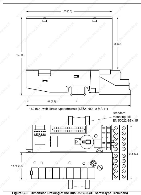
gure C-9. Dimension Drawing of the Bus Unit (SIGUT Screw-type Terminal with I/O Module
