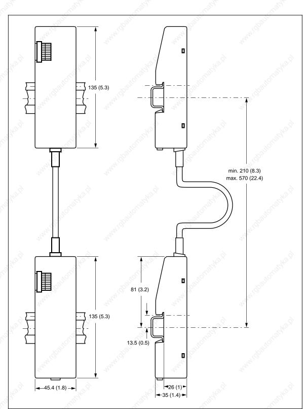
Figure C-11. Dimension Drawing of the IM 315 Interface Module
