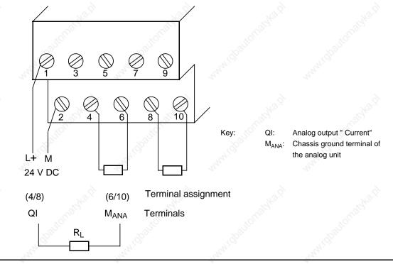
Figure 15-21. Connection via a Two-Wire Circuit (6ES5 470-8MC12)
