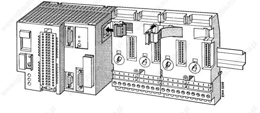
Figure 3-8. Connecting the Bus Units
