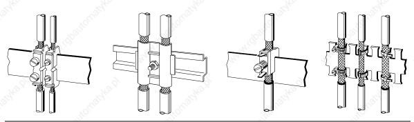
Figure 3-32. Fixing Shielded Cables with Various Types of Cable Clamps
