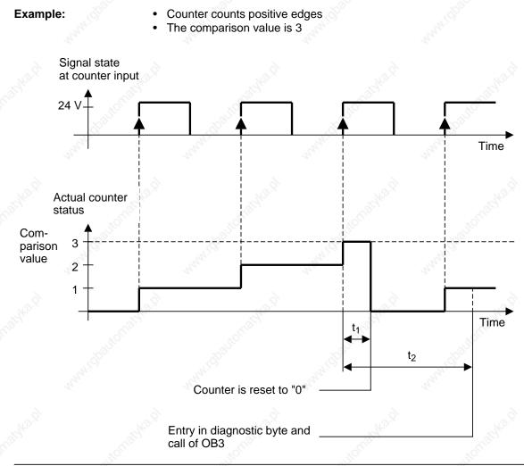
Figure 11-1. Principle of Operation of the Onboard Counter Inputs
