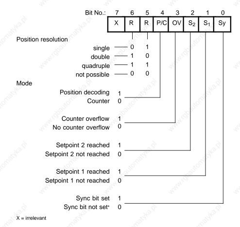
\* If the sync bit is not set, a reference point approach must be implemented before operation can continue in the "Position decoding" mode.
