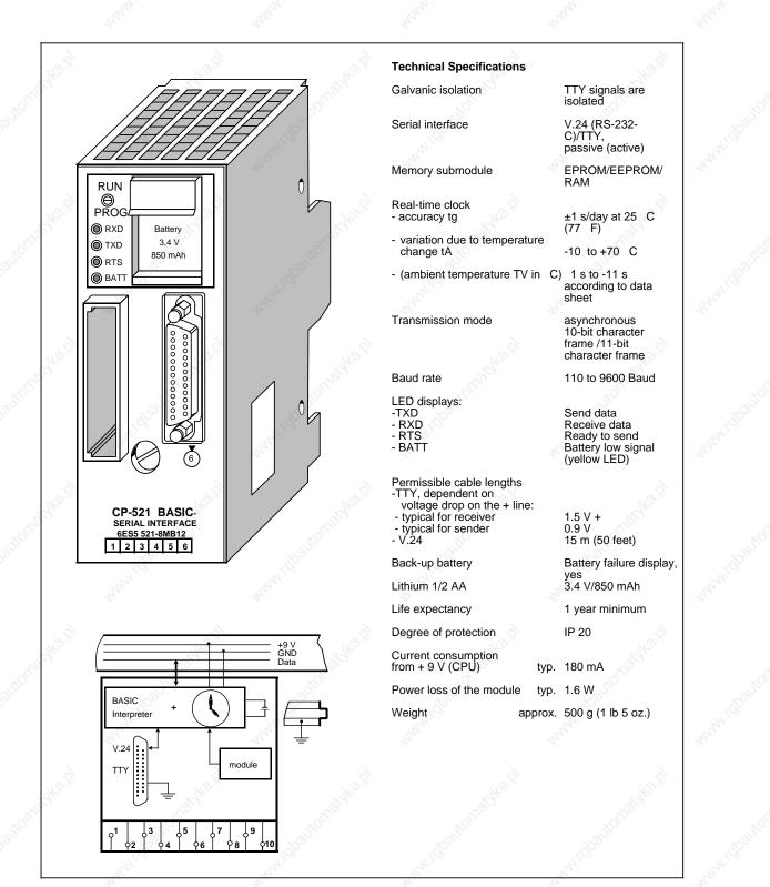
The CP 521 BASIC is a powerful peripheral module that can be used with the SIMATIC systems S5-90U, S5-95U and the S5-100U. It has its own central processor (cannot be used with the CPU 100, 6ES5 100-8MA01).
