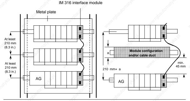
Figure 3-11. Minimum Clearances for a Multi-Tier Configuration Mounted in a Cabinet; PLC without/with Module Configuration/Cable Duct
