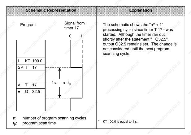
Except for "Reset timer", all timer operations are started only on an edge of the RLO. (The RLO alternates between "0" and "1".)
