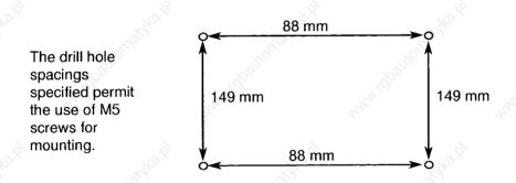
Figure 3-2. Drilling Template for Mounting the S5-90U Using Wall Brackets
