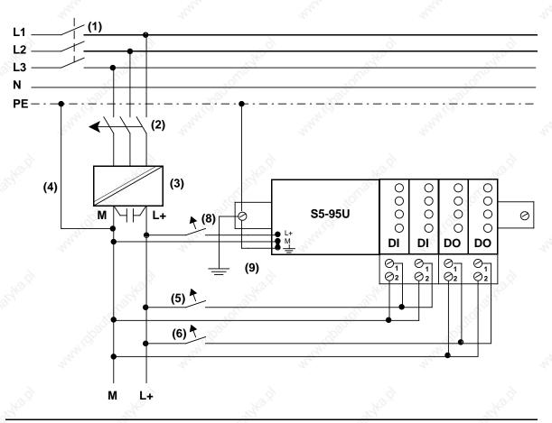
Figure 3-27. Grounded Configuration of the S5-95U with a 24 V DC Power Supply (with Safe Electrical Isolation in Accordance with DIN VDE 0160) for a Programmable Controller and Non-Floating, External I/Os
