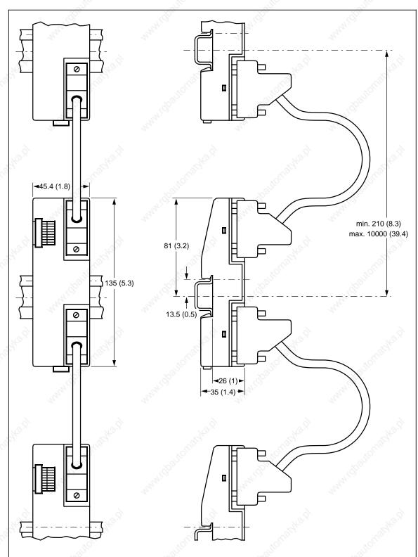
Figure C-12. Dimension Drawing of the IM 316 Interface Module
