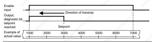
Figure 16-24. Approaching a Setpoint in Down-Count Direction
