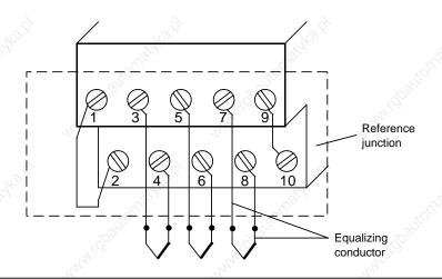
Figure 15-6. Remote Connection of Thermocouples of the Same Type with Linearization and Internal Compensation to the Module
