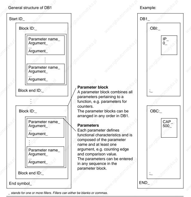
Figure 9-8. Structure of DB1
