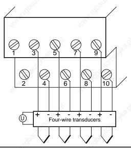
Figure 15-10. Connection of only Four-Wire Transducers (6ES5 464-8MD11)
