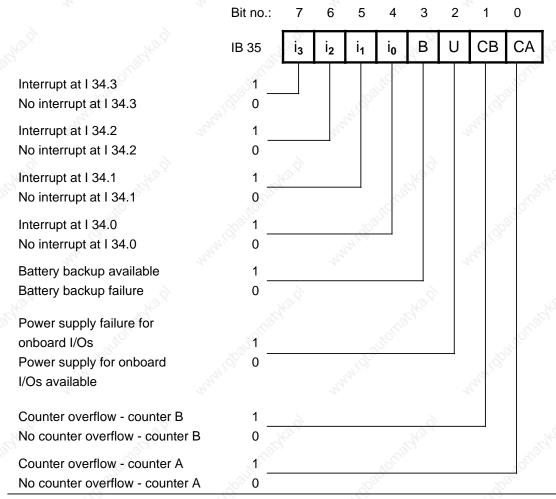
Figure 5-2. Diagnostic Byte for the S5-95U
