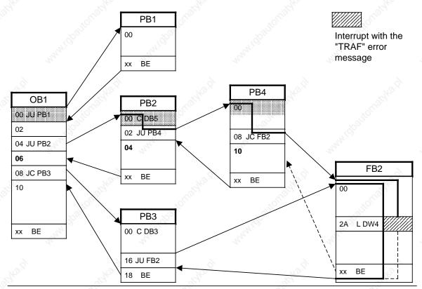
Figure 5-4. Program Tracing with "BSTACK"
