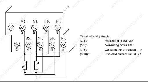
Figure 15-16. Wiring Method for PT 100 (6ES5 464-8MF11)
