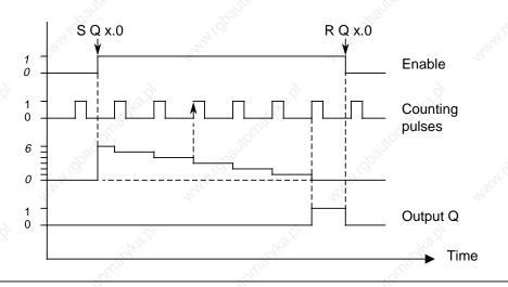
Figure 16-7. Timing Diagram: Setting and Resetting an Output of the Counter Module (500 Hz)
