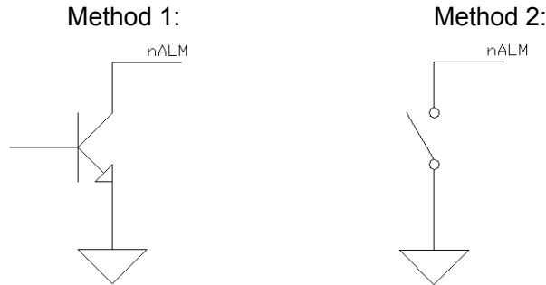
Fig. 2-1-4. Methods of the drive unit providing signals
