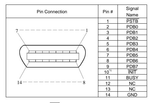
\*1 When not using the INIT signal, the 10 pin connection becomes unnecessary.
