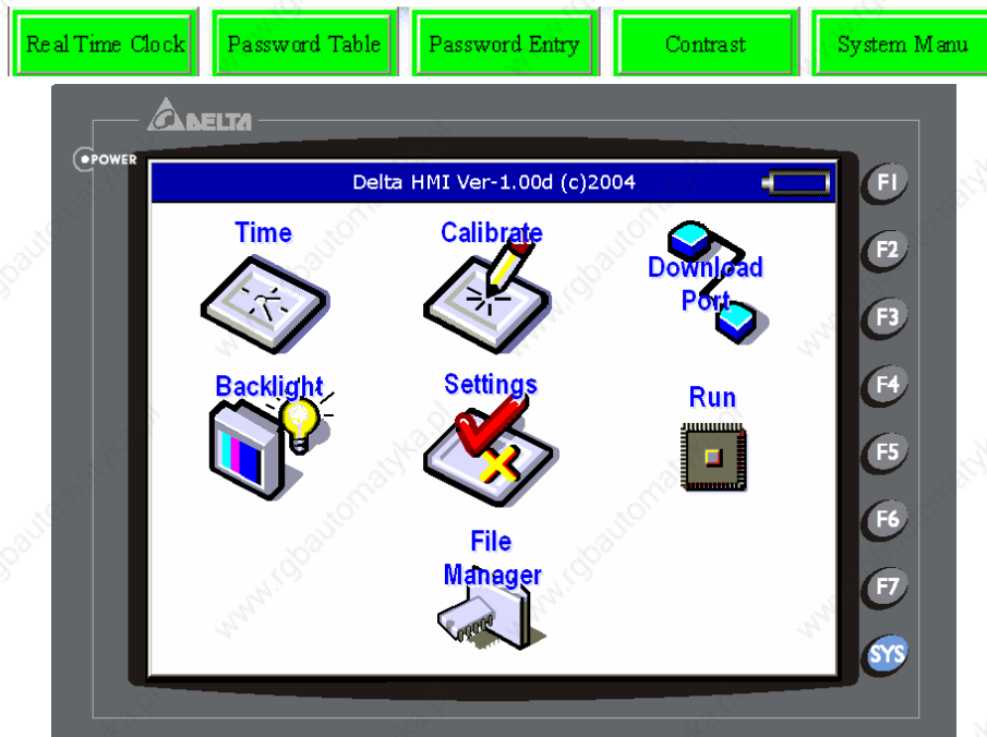
Fig. 3.2.8 HMI System Menu Screens
