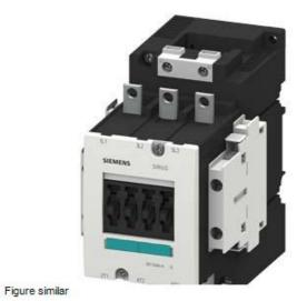
CONTACTOR AC-1, 140 A/400 V, 24 V DC, 3-POLE, SIZE S3, SCREW TERMINAL, WITHOUT BOX TERMINALS LATERAL AUX. SWITCH BLOCK L+ R 2 NO + 2 NC.
