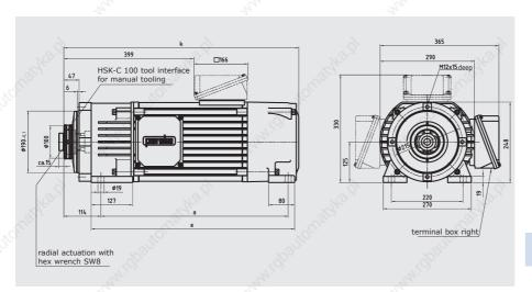
Type: KS 111 D Drawing: MS 630 C114 Shaft end: HSK-C100
