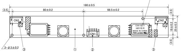
Oblique line portion in the upper figure shows silicone coating position.
