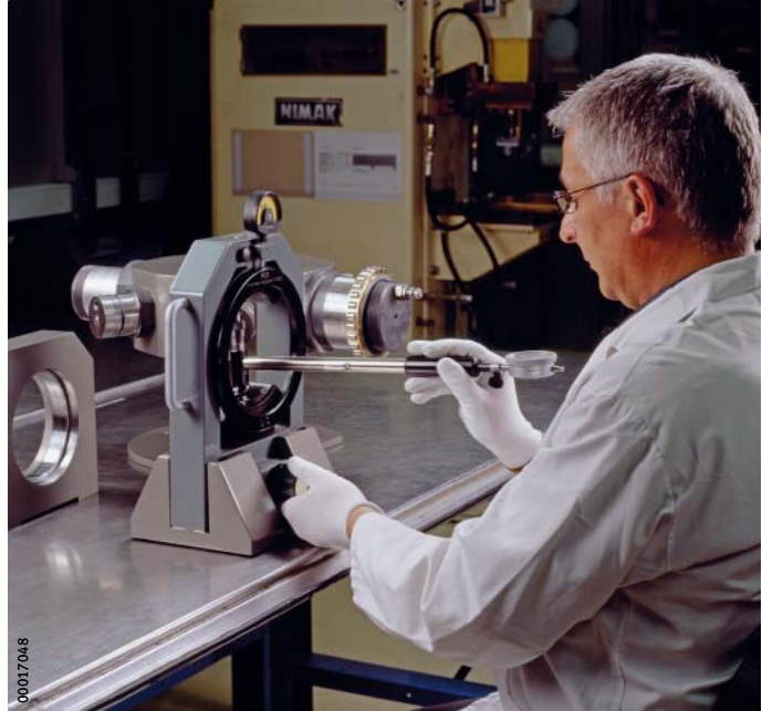
Figure 3 Transferring the raceway diameter to the enveloping circle gauge
