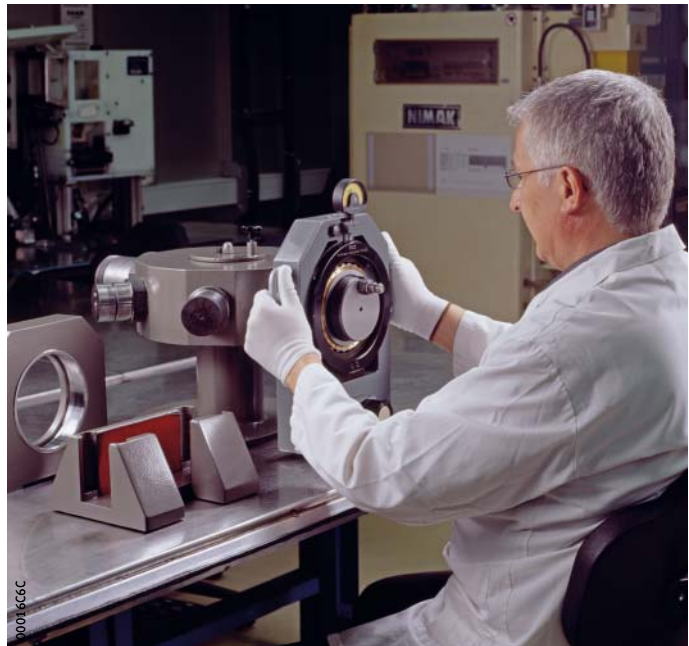
Figure 4 Positioning the enveloping circle gauge
