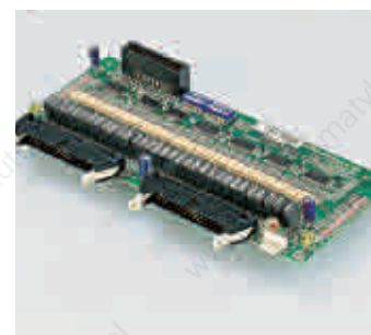
Output board 32 transistor outputs 0.8A
