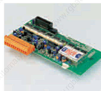
Analogue output board 2 outputs, 10bit resolution
