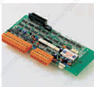
Analogue input board 4 inputs, 10bit resolution
