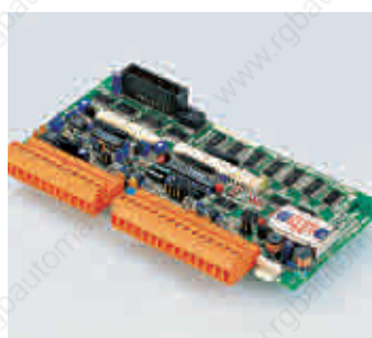
Analogue I/O board 4 inputs/1 output, 8bit resolution
