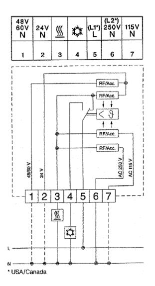
Contacts: Single-pole changer as a quick-break switch. Permissible contact data:
