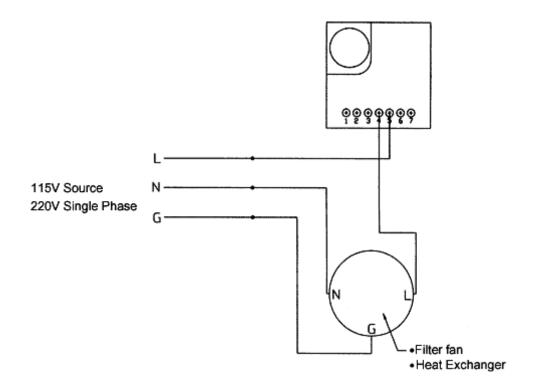
3110 Thermostat, wiring a panel heater:
