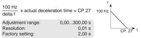
Example: actual deceleration time = 5s; the drive should decelerate from 50 Hz to 0 Hz, delta f = 50 Hz - 0 Hz = 50 Hz
