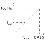
This function protects the frequency inverter against switching off through overcurrent during the acceleration ramp. When the ramp reaches the adjusted value, it is stopped so long until the current decreases again. CP.3 displays "LAS" at active function.
