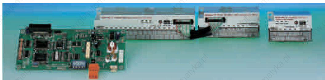
MEWNET TR sensor/actuator bus (master board and slave terminals)
