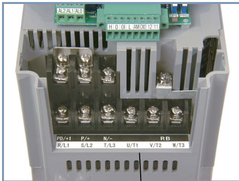
Power and motor connection terminals
