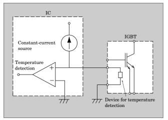
temperature for case protection, there is the possibility that the IGBT chips may be destroyed if this operating condition continues. It is clear that the device overheat protection function is indispensable.
