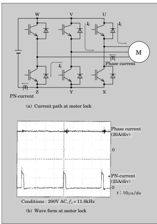
When the current was concentrated to the chip which was located on the far side from the sensor on the substrate, the sensor could not follow the rapid temperature risings and could not protect it. In order to solve these problems and to realize higher performance as well as higher cost performance, the R-IPM was developed.
