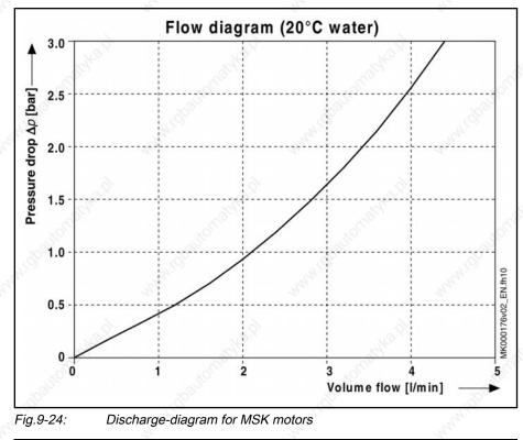
If a different coolant is used, a different coolant-specific flow diagram is applicable.
