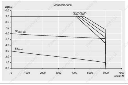
Mmax for IndraDrive, controlled feed, 3x AC 400V Mmax for IndraDrive, uncontrolled feed, 3x AC 480V Mmax for IndraDrive, uncontrolled feed, 3x AC 440V Mmax for IndraDrive, uncontrolled feed, 3x AC 400V Speed-torque characteristic of MSK050B-0600
