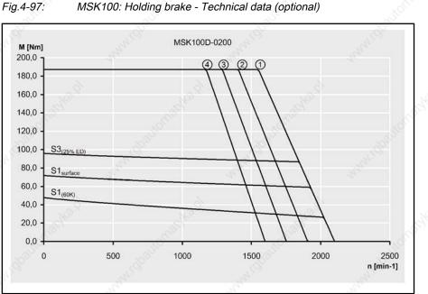
Mmax for IndraDrive, controlled feed, 3x AC 400V Mmax for IndraDrive, uncontrolled feed, 3x AC 480V Mmax for IndraDrive, uncontrolled feed, 3x AC 440V Mmax for IndraDrive, uncontrolled feed, 3x AC 400V Speed-torque characteristic of MSK100D-0200
