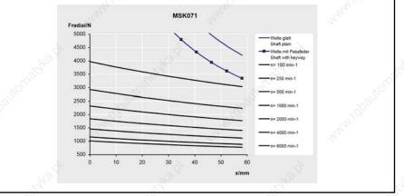
Fig.4-69:permissible radial force of MSK071 - Motors (shaft and bearing load)The maximum permissible axial force  $F_{axial}$  is 500 N.
