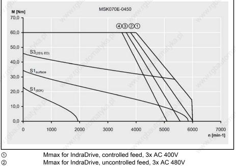
3 4 Fig.4-60: Mmax for IndraDrive, uncontrolled feed, 3x AC 480V Mmax for IndraDrive, uncontrolled feed, 3x AC 440V Mmax for IndraDrive, uncontrolled feed, 3x AC 400V Speed-torque characteristic of MSK070E-0450
