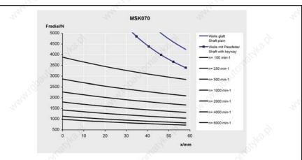
Fig.4-55:permissible radial force of MSK070 - Motors (shaft and bearing load)The maximum permissible axial force  $F_{axial}$  is 500 N.
