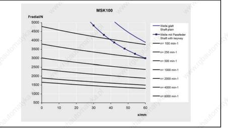
Fig.4-89:permissible radial force of MSK100 - Motors (shaft and bearing load)The maximum permissible axial force  $F_{axial}$  is 500 N.
