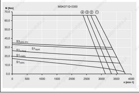
Mmax for IndraDrive, controlled feed, 3x AC 400V Mmax for IndraDrive, uncontrolled feed, 3x AC 480V Mmax for IndraDrive, uncontrolled feed, 3x AC 440V Mmax for IndraDrive, uncontrolled feed, 3x AC 400V Speed-torque characteristic of MSK071D-0300
