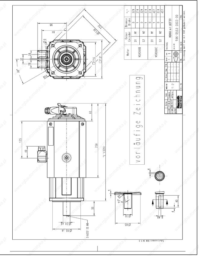
Fig.7-7: Dimension sheet MSK060 with axial fan unit
