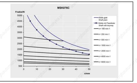
$\label{eq:Fig.4-82:} \textit{permissible radial force of MSK076 - Motors (shaft and bearing load)} \\ \text{The maximum permissible axial force $F_{axial}$ is $200 $N$} .$
