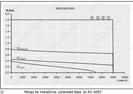
Mmax for IndraDrive, uncontrolled feed, 3x AC 480V Mmax for IndraDrive, uncontrolled feed, 3x AC 440V Mmax for IndraDrive, uncontrolled feed, 3x AC 400V Speed-torque characteristic of MSK030B-0900
