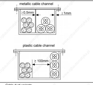
Fig.8-40: Cable duct variants
