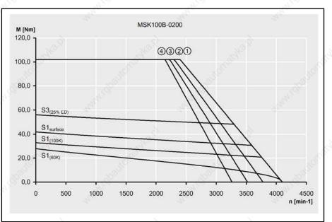
Mmax for IndraDrive, controlled feed, 3x AC 400V Mmax for IndraDrive, uncontrolled feed, 3x AC 480V Mmax for IndraDrive, uncontrolled feed, 3x AC 440V Mmax for IndraDrive, uncontrolled feed, 3x AC 400V Speed-torque characteristic of MSK100B-0200
