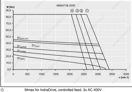
Mmax for IndraDrive, controlled feed, 3x AC 400V Mmax for IndraDrive, uncontrolled feed, 3x AC 480V Mmax for IndraDrive, uncontrolled feed, 3x AC 440V Mmax for IndraDrive, uncontrolled feed, 3x AC 400V *Speed-torque characteristic of MSK071E-0200*
