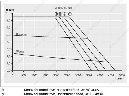
Mmax for IndraDrive, uncontrolled feed, 3x AC 480V Mmax for IndraDrive, uncontrolled feed, 3x AC 440V Mmax for IndraDrive, uncontrolled feed, 3x AC 400V Speed-torque characteristic of MSK050C-0300
