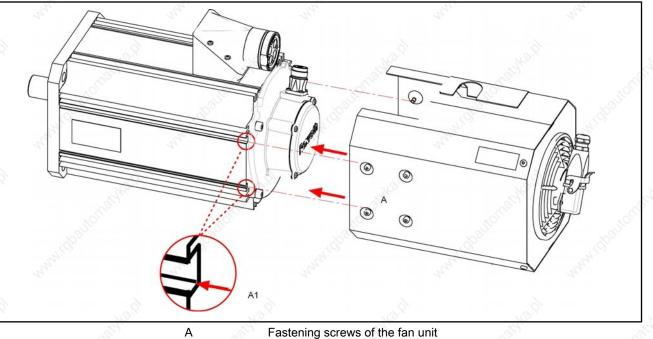
A A1 *Fig.7-13:*  Insert the fastening rail into the motor
