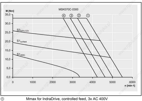
Mmax for IndraDrive, uncontrolled feed, 3x AC 480V Mmax for IndraDrive, uncontrolled feed, 3x AC 440V Mmax for IndraDrive, uncontrolled feed, 3x AC 400V Fig.4-47: Speed-torque characteristic of MSK070C-0300
