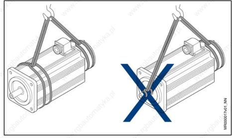
Fig.10-4: Lifting and transporting motors by means of lifting sling belts
