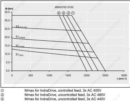
4 Fig.4-46: Mmax for IndraDrive, uncontrolled feed, 3x AC 440V Mmax for IndraDrive, uncontrolled feed, 3x AC 400V Speed-torque characteristic of MSK070C-0150
