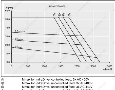
4) Fig.4-52: Mmax for IndraDrive, uncontrolled feed, 3x AC 440V Mmax for IndraDrive, uncontrolled feed, 3x AC 400V Speed-torque characteristic of MSK070D-0150
