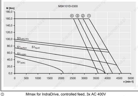
Mmax for IndraDrive, controlled feed, 3x AC 400V Mmax for IndraDrive, uncontrolled feed, 3x AC 480V Mmax for IndraDrive, uncontrolled feed, 3x AC 440V Mmax for IndraDrive, uncontrolled feed, 3x AC 400V Speed-torque characteristic of MSK101D-0300
