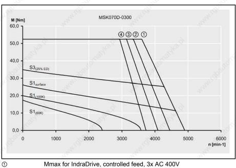
Mmax for IndraDrive, uncontrolled feed, 3x AC 480V Mmax for IndraDrive, uncontrolled feed, 3x AC 440V Mmax for IndraDrive, uncontrolled feed, 3x AC 400V Fig.4-53: Speed-torque characteristic of MSK070D-0300
