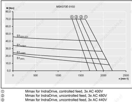
4) Fig.4-58: Mmax for IndraDrive, uncontrolled feed, 3x AC 400V Mmax for IndraDrive, uncontrolled feed, 3x AC 440V Mmax for IndraDrive, uncontrolled feed, 3x AC 400V Speed-torque characteristic of MSK070E-0150
