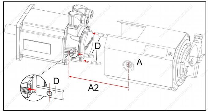
*Fig.7-12:* Assembly of fan unit LEM-AB-116N-xx-NNNN Mounting procedure
