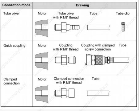
Fig.8-42: Connection variants liquid cooling
