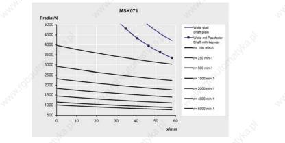
$\label{eq:Fig.4-77:} \textit{permissible radial force of MSK071 - Motors (shaft and bearing load)} \\ \text{The maximum permissible axial force $F_{axial}$ is $500 $N$} \, .$
