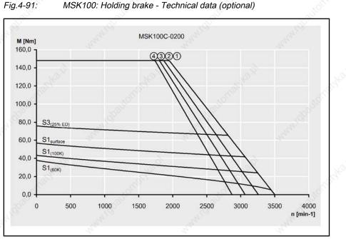
1) 2) 3) 4) Fig.4-92: Mmax for IndraDrive, controlled feed, 3x AC 400V Mmax for IndraDrive, uncontrolled feed, 3x AC 480V Mmax for IndraDrive, uncontrolled feed, 3x AC 440V Mmax for IndraDrive, uncontrolled feed, 3x AC 400V Speed-torque characteristic of MSK100C-0200
