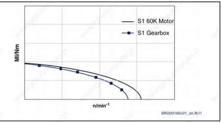
Fig.9-19: S1 characteristic curve of gearboxes
