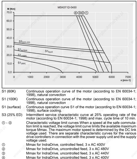
Example of a motor characteristic curve
