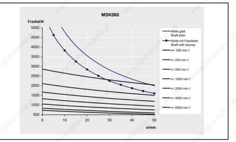
$\label{eq:Fig.4-34:} \textit{permissible radial force of MSK060 - Motors (shaft and bearing load)} \\ \text{The maximum permissible axial force $F_{axial}$ is $350 N$.}$
