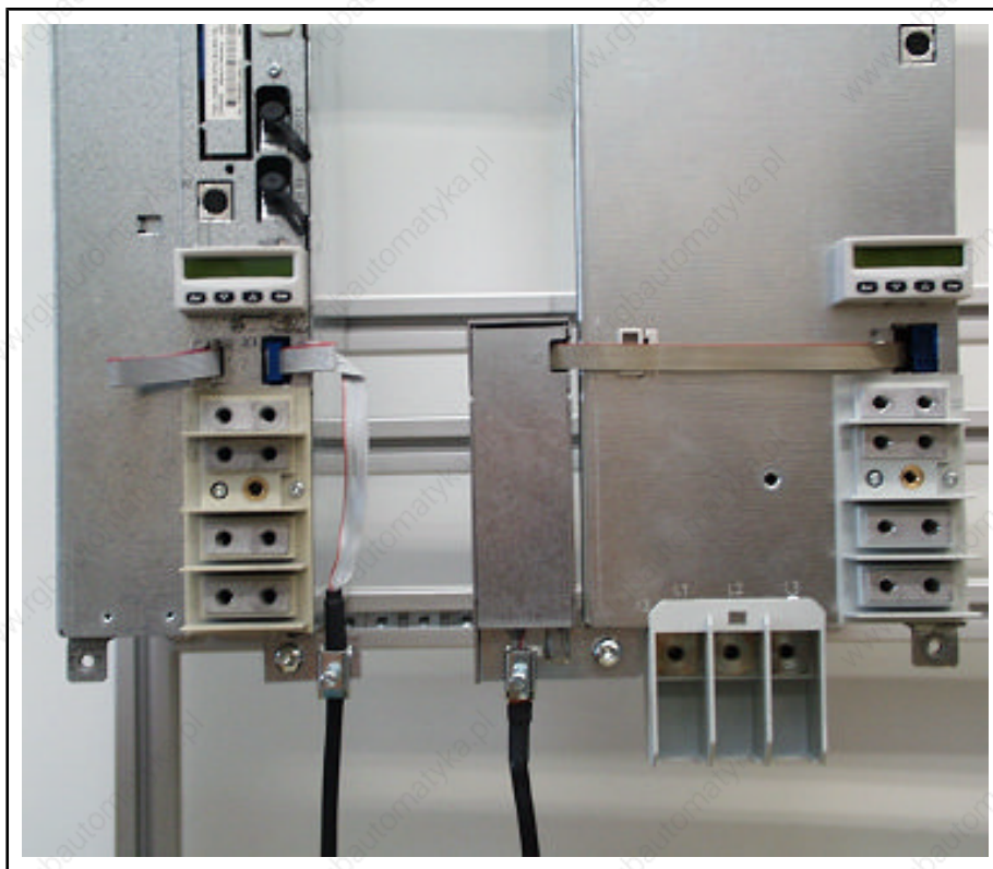
Fig. 14-140: Extension of module bus
