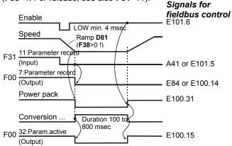
When autostart is active (**A34**=1), the switchover takes place immediately when the edge of the signal "*11:Paraset*" occurs. Enabling is automatically deactivated internally.
