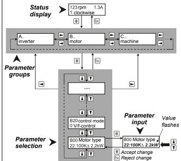
After power-on, the inverter only shows the most important parameters which are required for commissioning. To solve complex drive tasks:
