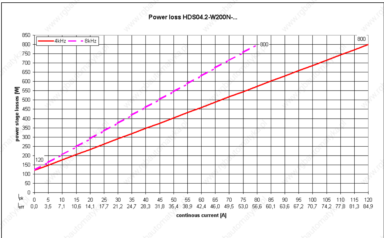
Fig. 7-5: Power loss HDS04.2W0200N-
