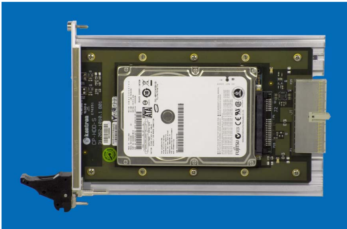
Figure 2-3: CP-HDD-S Carrier Board With HDD Mounted
