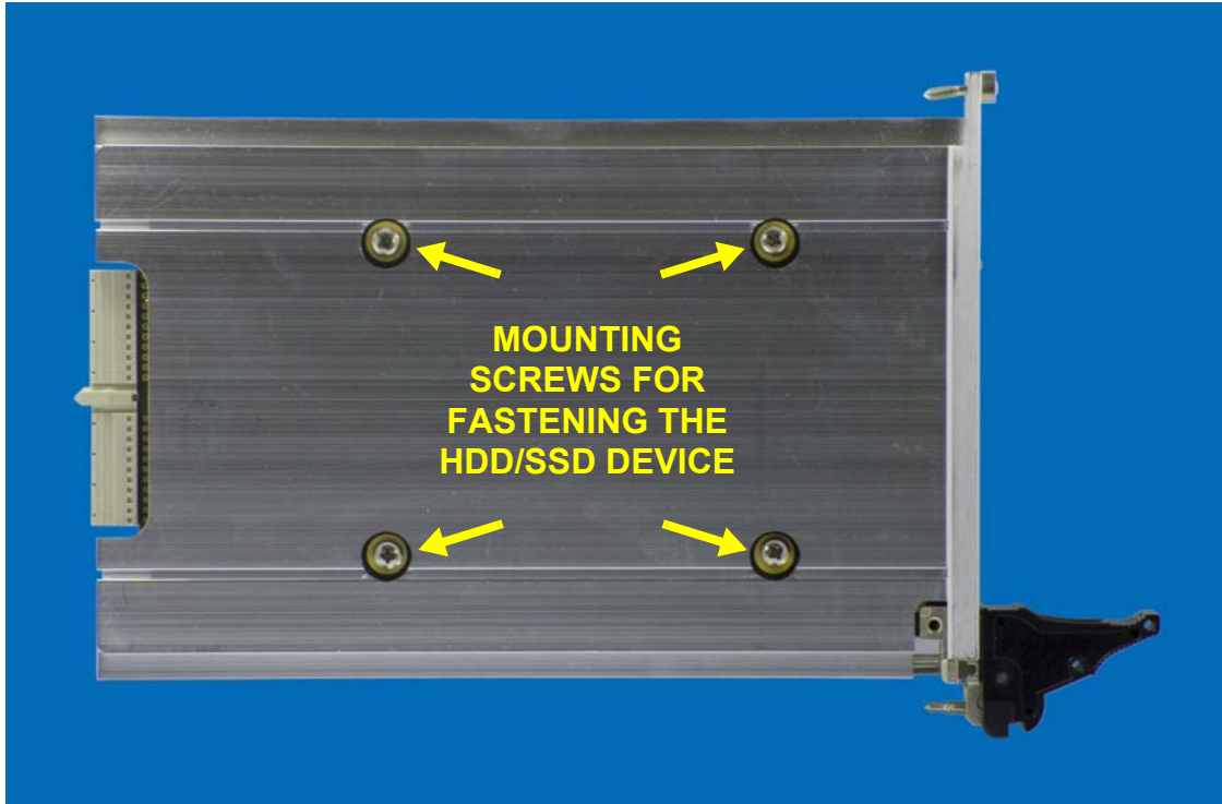
Figure 2-3: CP-HDD-S Carrier Board With HDD Mounted
