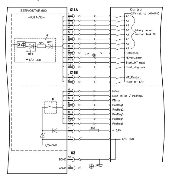
**NOTE** AGND and DGND (connector X3) must be joined together!
