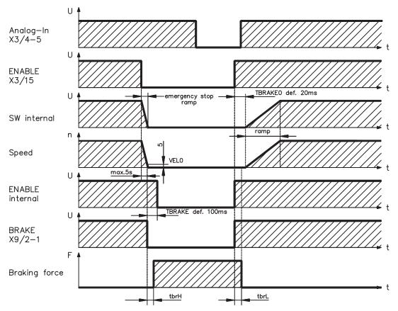
During the internal ENABLE delay time of 100ms (DECDIS) the speed setpoint of the servo amplifier is internally driven down a 10ms ramp to 0. The brake output is switched on when the speed 5rpm (VELO) is reached or after 5s (EMRGTO) the latest.
