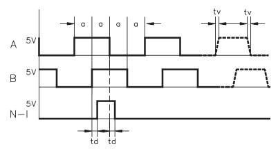
Edge spacing a  $\geq$  0,20  $\mu s$ Edge steepness tv  $\leq$  0.1  $\mu s$ Delay N-I-td  $\leq$  0.1  $\mu s$  $I\Delta UI \geq 2V/20 mA$
