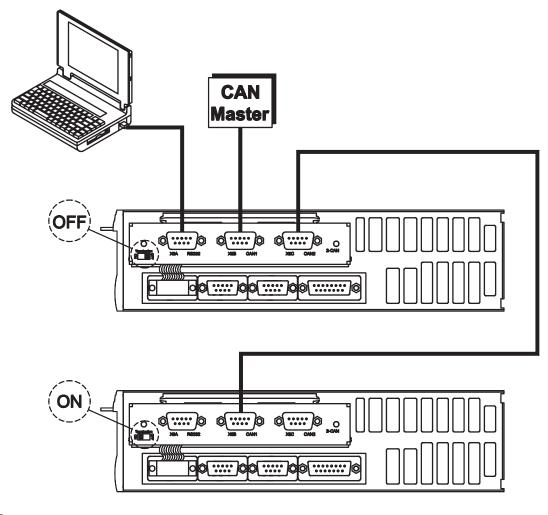
NOTE AGND and DGND (connector X3) must be joined together!
