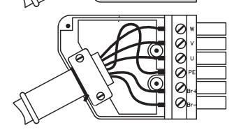
Place the connector in the housing. Take care that the tongue of the shield plate sits in the PE clamp. Wire up the connector according to the wiring diagram on page 50, and tighten up the clamping screws. Take care that the insulation is not trapped underneath. Close the housing.
