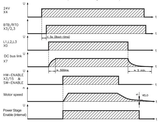
Devices which are equipped with a selected "Brake" function use a special sequence for switching off the output stage (⇒ p.26).
