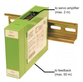
The extended power supply enables the operation of encoder systems at connector X1 with a power consumption of up to 400 mA DC. This power supply is switched between X1 and the encoder and supplied by SERVOSTAR 600.
