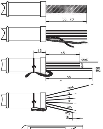
First push the rubber sleeve onto the cable, and **then** strip off about 70mm of the outer covering, without damaging the shielding.
