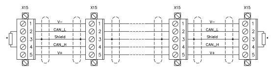
\* according to line impedance about  $120\,\Omega$
