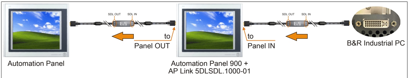
Figure 131: Example of the signal direction for an SDL flex cable with extender
