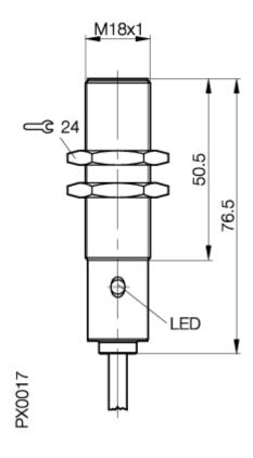
Inductive Sensors BES 516-326-BO-H M18x1 x 76.5 normally-open Sn=5mm shielded
