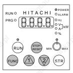
(1) Hold down the FUNC, UP and DOWN key and then press the STR key. When the display starts to flash and rotate release all the keys.
