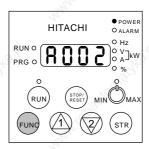
The changed set value is confirmed by pushing the STR key.
