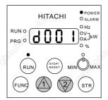
Monitor mode is displayed by pushing FUNC (Function) key once when display of Monitor mode No.
