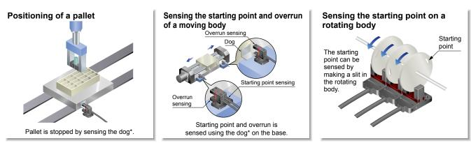
\*"Dog" refers to the sensing object for activating the sensor's detecting operation.
